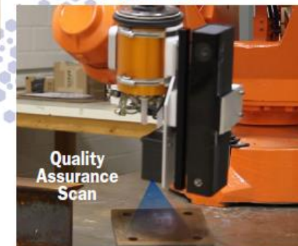
Figure 4: After blending, the system executes a quality assurance scan with a high resolution laser line scan sensor.
